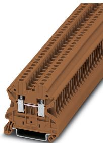
Feed-through terminal block, nom. voltage: 1000 V, nominal current: 24 A, connection method: Screw connection, number of connections: 2, cross section: 0.14 mm<sup>2</sup> - 4 mm<sup>2</sup>, AWG: 26 - 12, width: 5.2 mm, color: brown, mounting type: NS 35/7,5, NS 35/15
