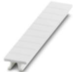
Zack marker strip, can be ordered: Strip, white, labeled according to customer specifications, mounting type: snap into tall marker groove, for terminal block width: 5.2 mm, lettering field size: 5.15 x 10.5 mm, Number of individual labels: 10
